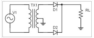
For this circuit, you need to remember that only half of the secondary's voltage appears at the output at any given time -- the other half of the secondary can't conduct when its diode is reverse-biased.
